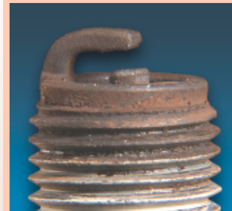
After 500 hours of runtime with STIHL HP Ultra oil, this spark plug is in excellent shape.
