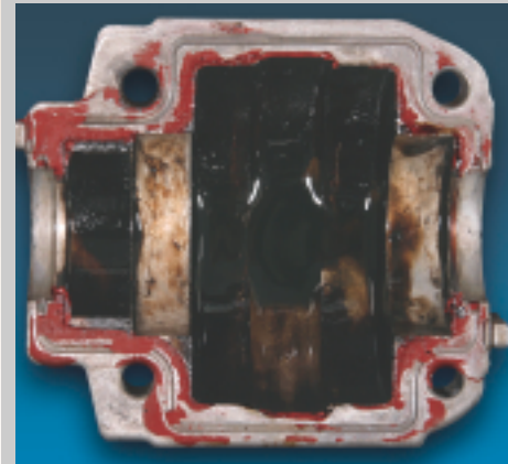
Extreme buildup of damaging particles and sludge cover the inside of this crankcase with Competitor B oil.
