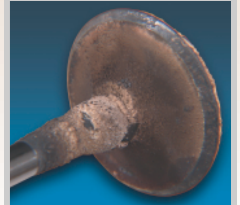
Excessive buildup on this valve from Competitor B oil can cause loss of power and performance.
