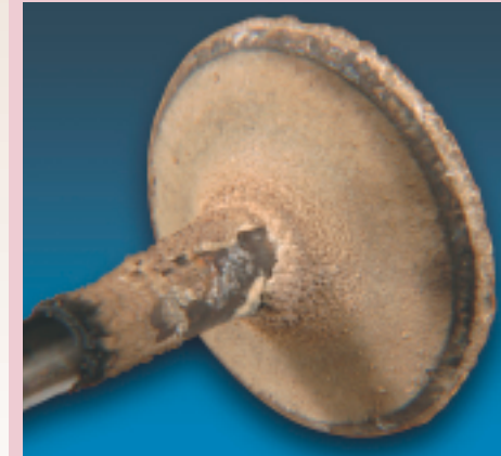
Excessive carbon buildup on this valve from Competitor A oil prevents heat dissipation.
