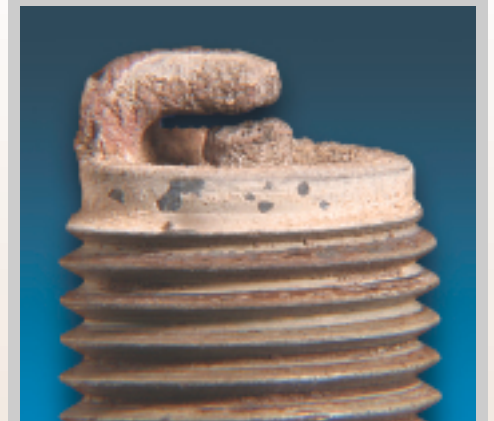
This heavily fouled spark plug from using Competitor B oil will cause it to misfire.
