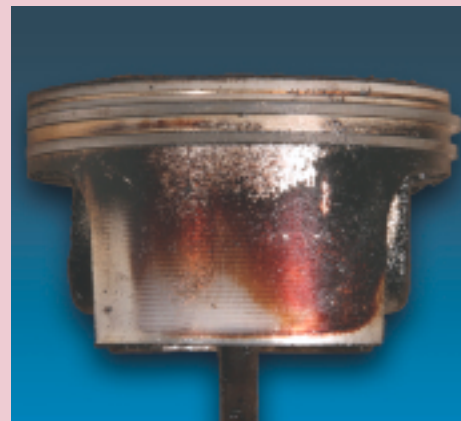
This piston from Competitor A oil has major particle and sludge buildup to cause engine damage.
