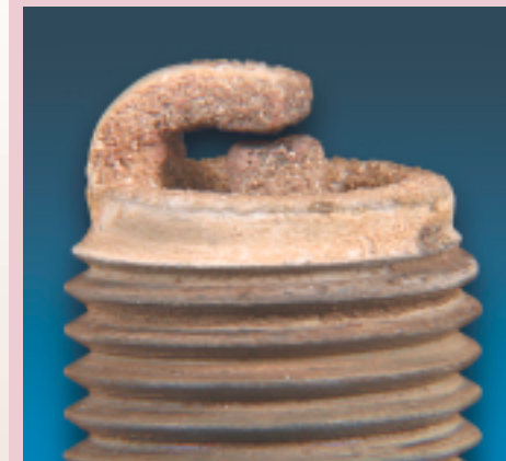
This fouled spark plug from Competitor A oil will ground out rather than fire normally.
