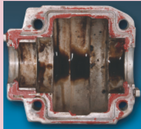
This crankcase with Competitor A oil has excessive damaging particles and sludge.
